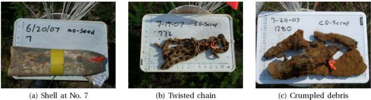
Figure 3.30: a) Unexploded shell from Cell No. 7 and (b,c) the two false alarms obtained by the SVM classifier using k and as discriminators.
